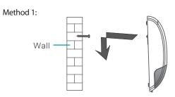
A. Mark drill hole and drillon the wall.
