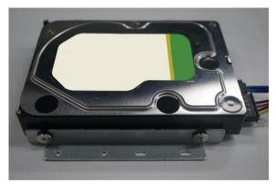
4. Connect one end of the data cable and power cable to the hard disk.
