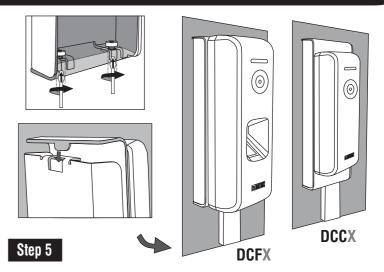
Fix Top Cover to Base Plate by sliding Mounting Hook of top cover into the Mounting Slot of base plate. Tighten screws at the bottom as shown.
