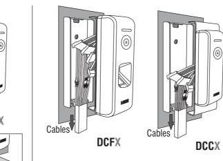
Connect cables and lead cables Step 4 through bottom opening of Duct Box
