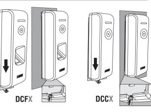
Step 4 When in place, tighten captive screw at bottom
