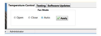
When use Temp. Control, you can choose "Auto" to recognize temperature automatically or "Manualsetting" to set the RunValue & StopValue, or choose "Open" / "Close" to keep on /off status, multiple combination provide much convenience for users.
