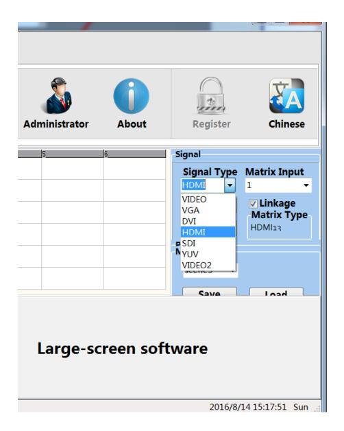
(3)If have matrix, with  $\sqrt{\ }$  in the matrix linkage can choose to display matrix output channel. Specific settings with reference to the matrix description.
