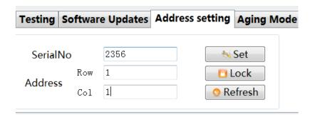
input 2356 in SeralNo., 1 in Row, 1 in Col and click Set button, "Address set successfully" will be displayed on the screen 1,then click the Lock button,the address will be locked.
