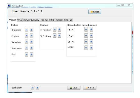
Adjustment range: selected coordinate unit area of the current operating area. All parameter adjustments will be effective in the selected cell area.
