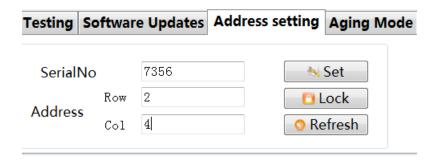
input 7356 in SeralNo., 2 in Row, 4 in Col and click Set button, "Address set successfully" will be displayed on the screen 8,then click the Lock button, the address will be locked.
