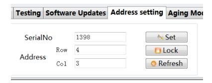
input 1398 in SeralNo., 4 in Row, 3 in Col and click Set button, "Address set successfully" will be displayed on the screen 15, then click the Lock button, the address will be locked.
