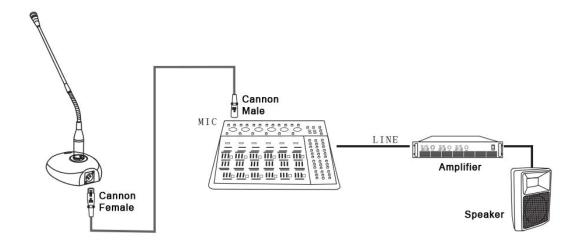
B: Connect the microphone to audio console
