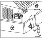
3. For disarm, press the key DISARM for 2 seconds.
